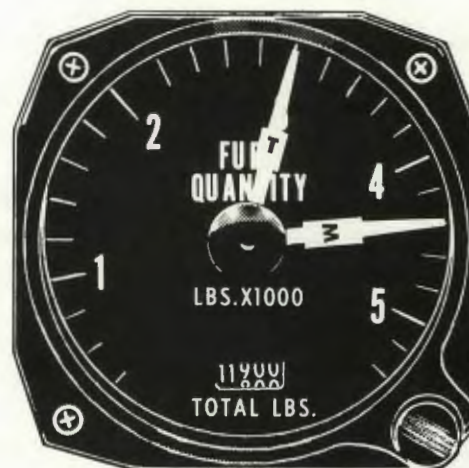
2. In the same situation (fuel in the externals), if the "T" needle begins to move (decrease in quantity) it is an indication that the externals are not feeding. A quick check with the fuel tank quantity monitoring switch will confirm your suspicions.
