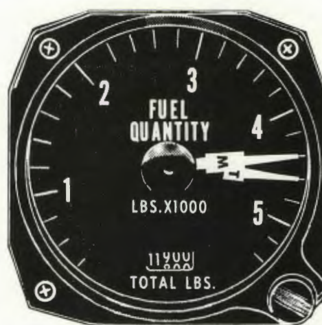
1. While in flight with the fuel tank quantity monitoring switch in "wing" position and fuel in the external tanks, the "M" and "T" needles would be in these approximate positions. Under normal feed conditions the "T" needle would not move until the externals were empty.
